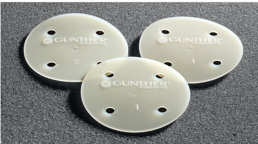
Fig. 5. Shot-weight 3 g, diameter 60 mm, wall thickness 1 mm; the “disk” test sample.
